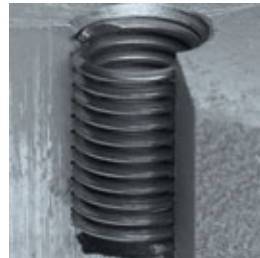
Cast aluminium component. Completely lined thread at small tap hole depth.
