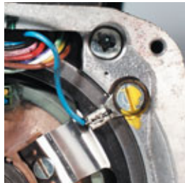
Controller. Three-phase servo motor with electronic positioning unit. Loose tangs would result in faults.
